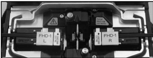
2: Place the fiber holder onto the fiber holder stage, fitting the pin of the stage into the hole of the fiber holder.
