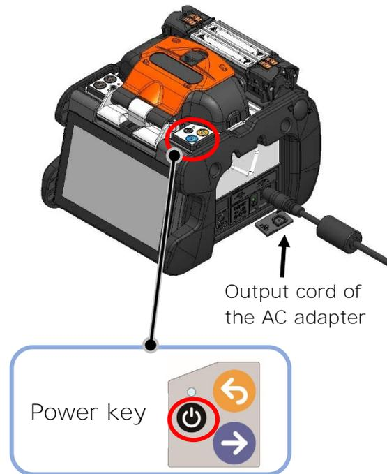
If you press the Power key right after connecting the power cord to the power supply module, it may take a few seconds until the splicer is powered on.
