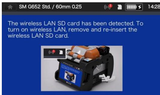
3: After the setup is complete, wireless LAN icon (
