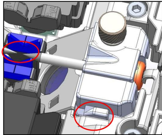
The protrusion does not fit in the splicer.
