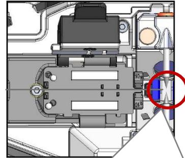
2: Place the fiber in the splicer so the fiber end is between the edge of the v-groove and the electrodes.
