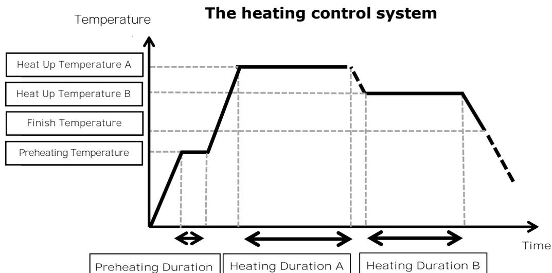
The heating control system is individually applied to each heater.
