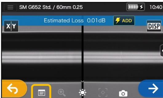
1: After splicing, tap the Splice data details icon (
