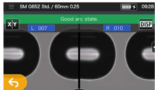
5: After "Good arc state." displayed, begin the fiber preparation procedure to perform a splice.
