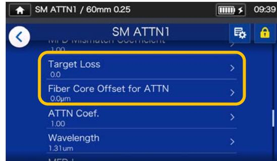
3: Select "Target Loss" or "Fiber Core Offset for ATTN" to edit the value.
