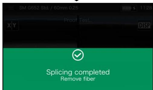
**When the proof test is complete, the screen as shown above is displayed.** ▶ Proceed with the heating process. See the next page.
