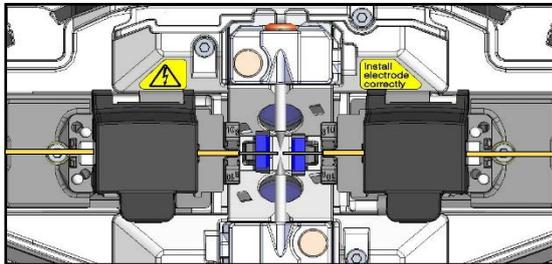
1: As mentioned in the previous pages, load a prepared fiber. (The coating is removed and fiber is cleaved.)
