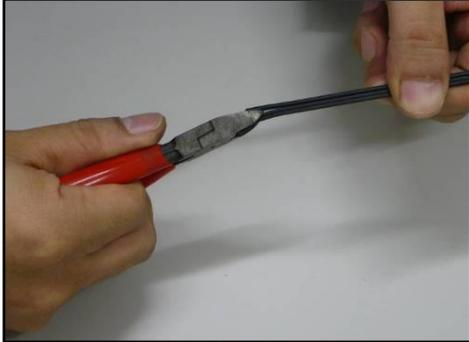
1: Separate the steel wire from the cable using nippers.
