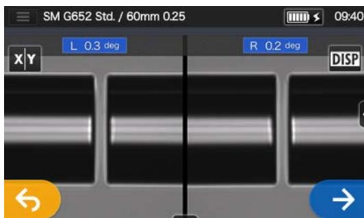
2: Inspection of fiber end face & dust.
