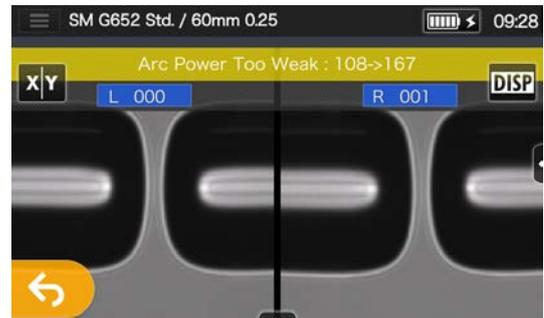
4: The melt back distance of the left and right fibers and the arc center position which are measured via image processing are displayed on the monitor screen. (The arc center position value is displayed only if the position is shifted.)
