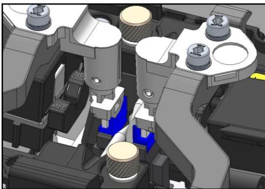
Make sure the bare fiber pad clamps the fiber properly.
