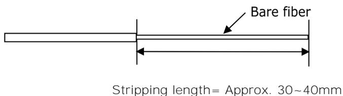
Use the correct groove of the remover according to the fiber coating diameter.
