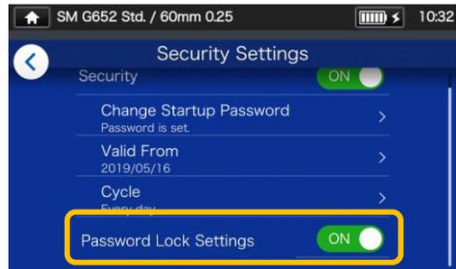
4: In Operator mode, splice program, heater program, function settings and sound setting cannot be edited.
