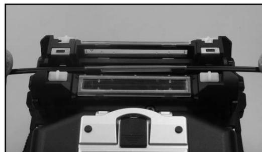
To keep excellent splice quality, regular cleaning and inspection are required. Especially cleaning should be performed before and after each use. We recommend your splicer to be checked through our maintenance service periodically.
