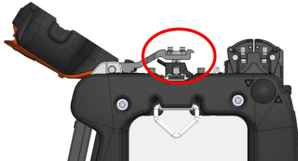
When the hood is opened, the bare fiber pad is detached from the hood.
