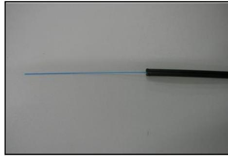
6: The cable sheath is removed. Repeat step 1 to 5 for the other cable. Cut each half of the cable sheath to the same length.
