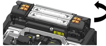
2: Open the hood and the fiber coating clamps. Take out the spliced fiber.
