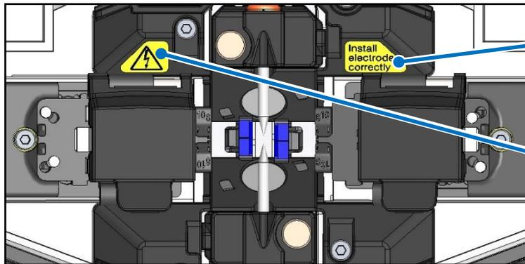
1 Installing electrode
