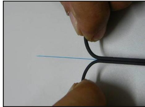
5: Split the cable sheath to expose 30~40mm of optical fiber. Cut off the split cable sheath.
