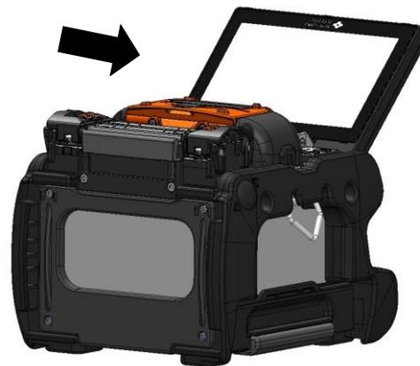
When the monitor is in the back position, your splicing work is easier if the right-hand and left-hand coating clamps are swapped. Refer to the following procedures.
