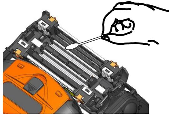
2: Clean the clamps of the heat shrink oven with a cotton swab moistened with alcohol.
