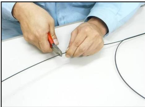
2: Cut the steel wire to a desired length.
