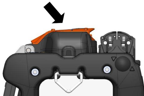
When the hood is closed, it catches the bare fiber pad. The hood and fiber pads are moved together.
