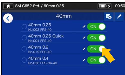
2: Tap  ON  OFF to switch between ON ↔ OFF.
