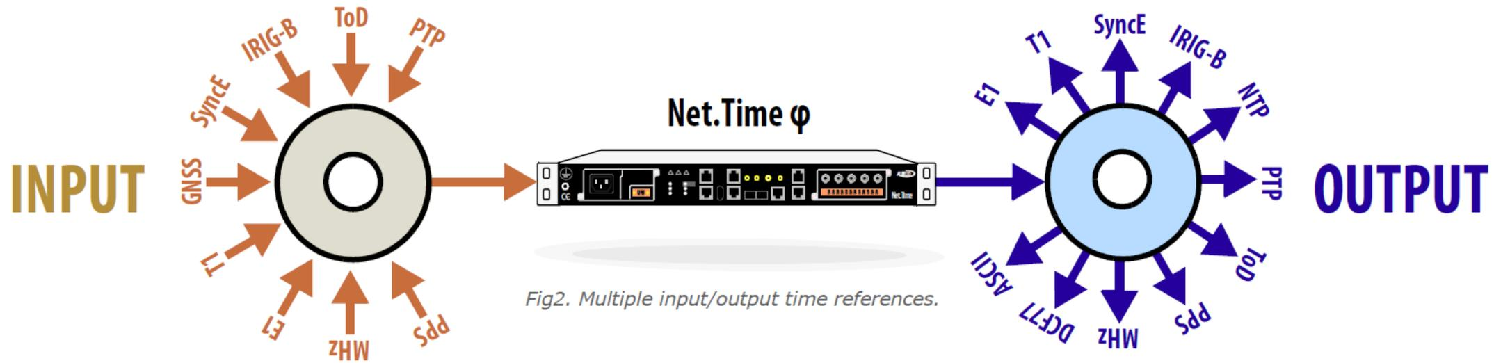
Net.Time is very flexible because it accepts multiple clock references to discipline the internal circuits. GNSS is the default and the most obvious reference but signals such as PTP, NTP, SyncE, ToD, IRIG-B even MHz, E1/T1 can also be used as back-up time references in case of failure of the first reference or in case of GNSS spoofing.
