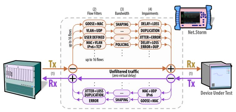
Net. Storm in operation: (1) connect in through mode, (2) program flow filters, (3) characterize bandwidth, (4) select impairments.
