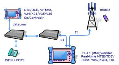
are often transported by T1, E1 lines. For instance, audio codec's like the G729 very popular in WANs, uses T1, E1 to handle up to 107 simultaneous calls interconnecting the new voice solutions by means of TDM circuits.
