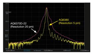
Spectrum of External Cavity Laser
