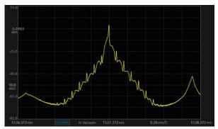
Modulated spectrum of 10G optical transceiver
