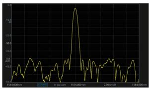
Transmission spectrum of optical filter
