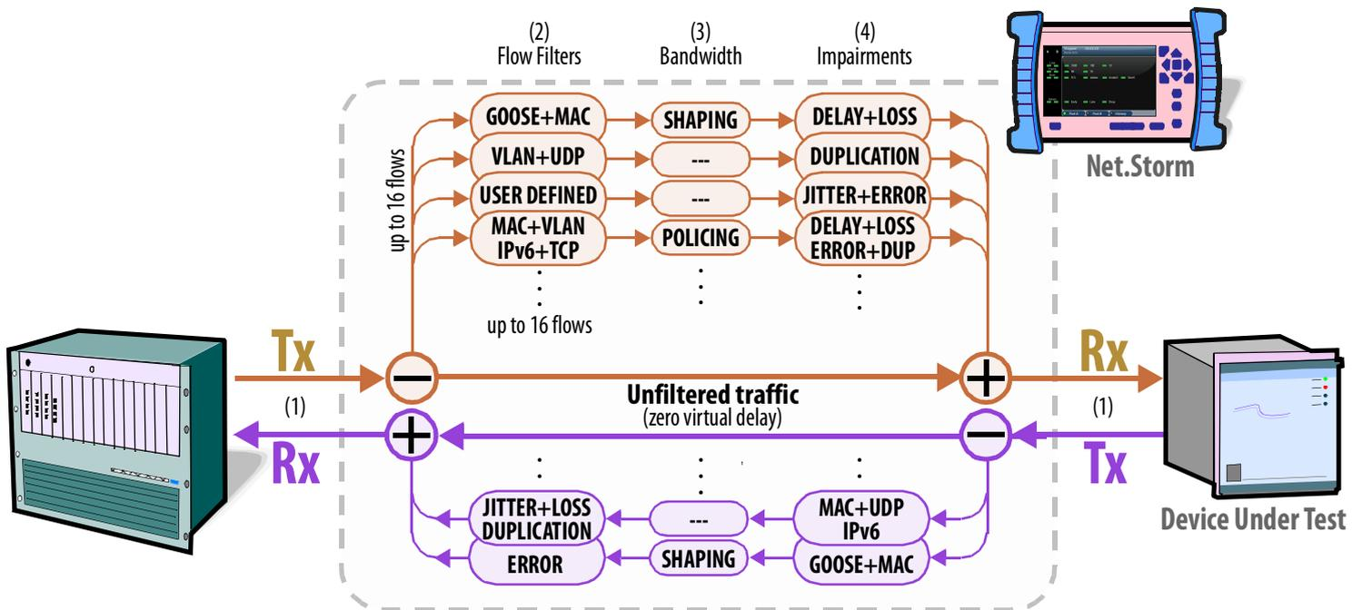
Net.Storm in operation: (1) connect in through mode, (2) program flow filters, (3) characterize bandwidth, (4) select impairments.
