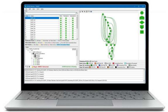
*Solution for monitoring and commissioning a GOOSE installation, consisting of a Tap and a Protocol Analyser. The Tap filters and forwards messages to GOOSE Monitor, the application that displays the IED topology and the messages in real time.*
